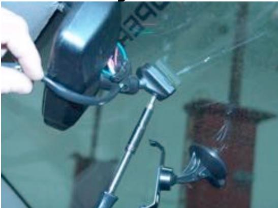
40. If the vehicle mirror is retained with a clip, use Mirror Removal Tool # OTC8200 available from Brandmotion.com or Ford dealers to release the mirror (Figure 17).
