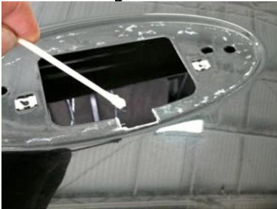
**18.** Route the camera harness through liftgate opening.
