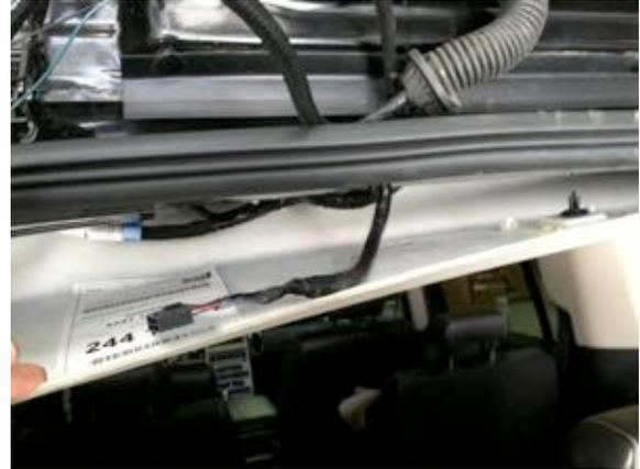
**25.** Route the light gray chassis harness camera connector end toward the light gray connector on the camera harness and connect (Figure 13).
