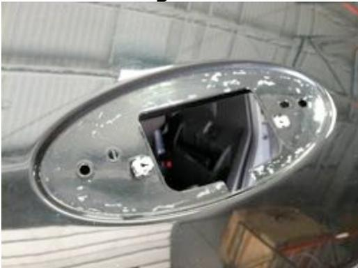
**13.** Mark, center punch, and drill a pilot hole for the camera mount harness opening (Figure 7). Using a 1 $\frac{3}{4}$  inch hole saw, cut the camera harness opening. Trial fit camera mount and file opening as necessary.
