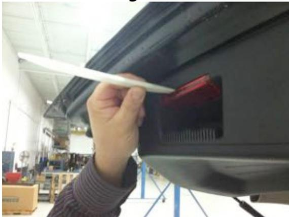
3. Unfasten the four screws with a Phillips screwdriver and pry up on the edges of the liftgate lower trim panel to release it from the liftgate. Remove liftgate lower trim panel and set aside (Figure 3).
