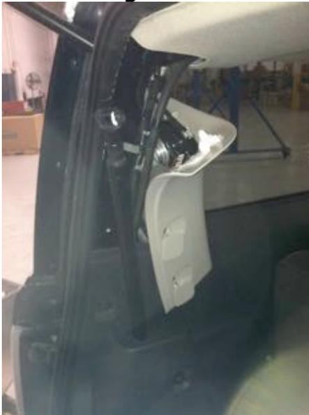
**23.** If necessary, use a razor knife to cut a small slit in the liftgate wiring grommet to assist in the routing of the chassis harness wiring through the grommet.
