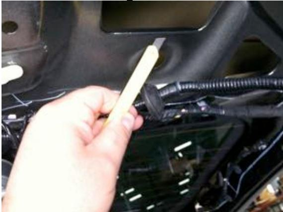
2. Raise liftgate. Using a plastic trim removal tool, pry off the two red plastic reflectors in the lower edge of the liftgate to expose four retaining screws (Figure 2).
