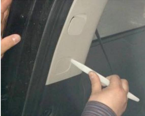
**22.** Remove the two bolts with a 7mm socket, and loosen the driver side upper D-pillar trim panel by peeling back weather stripping slightly and releasing the retaining clips (Figure 11).
