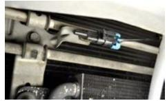
8. Route the sensor cable from the sensor and into the cabin area. Brandmotion recommends using an existing grommet and to avoid drilling through the firewall as there may be components/harnesses that could be easily damaged.
