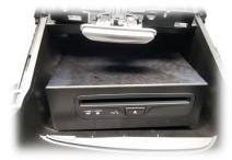
14. Leave sufficient slack in wire to allow bin to open and close without pinching or stretching wire.
