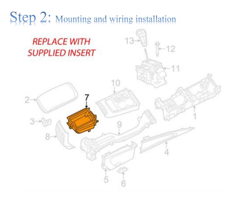
Disassemble factory center console to gain access to bin insert under armrest. Route extension harness from the T-Harness behind the radio to the location of the CD player, as pictured.
