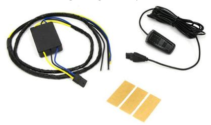
**Purpose**: This kit allows replacing the OE SYNC or Uconnect equipped mirror with built-in microphone with a Brandmotion Rear Camera Mirror while retaining full function of the SYNC or Uconnect system in the vehicle.
