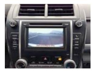
**Step 8: Reverse Feed (If Req'd)**. In Scion and Tacoma vehicles you may need to supply the reverse signal to the radio. Use the loose green wire supplied in this kit. First insert the terminal end into pin-2 of the white 28-pin radio connector. See page two of these instructions for your vehicle reverse wiring location.
