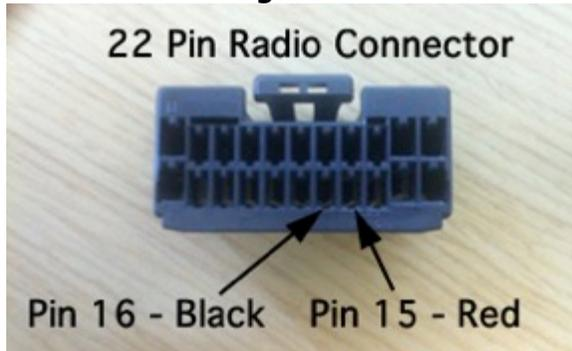
**IMPORTANT:** If the Gray 22-pin connector is present in the vehicle and Pins 15 and/or 16 are already populated, remove the terminal(s) using Delphi Terminal Removal Tool #12094429 or a Small Flat Watch Repair Screwdriver and isolate with Electrical Tape.
