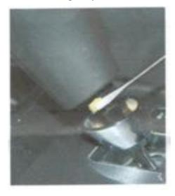
5. Use the plastic panel removal tool to gently lift on the sides of the shifter trim to unclip. Once removed disconnect the wiring harness from the under side.
