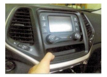
5. Remove the (4) Phillips screws that are holding in the radio to the dash. Remove the radio from the dash, disconnect all the harness from the back of the radio and set it side.
