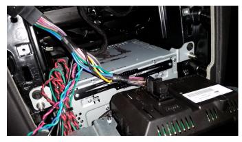
9. Then connect the opposite end to the vehicle harness, within 5 seconds turn the key to the run/ignition position. (Do not start the vehicle)
