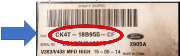
Next, confirm that your display part number appears in the COMPATIBLE display list below. INCOMPATIBLE part numbers are listed as well. (The example part number above appears in the COMPATIBLE list.) Please note: This is **NOT** a complete list of display part numbers, only displays that have been tested, as Ford can add new part numbers at any time.
