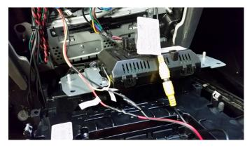
14. Mount module to top of radio/CD case in dash, behind screen.
