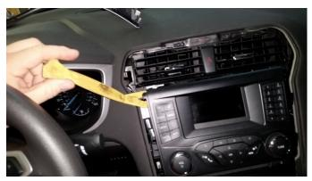
2. Remove the screws holding the screen into the dash.
