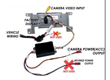
7. Disconnect the FCDIM/display harness on the back of the display by pushing down on the tab and pulling the "lever" back.
