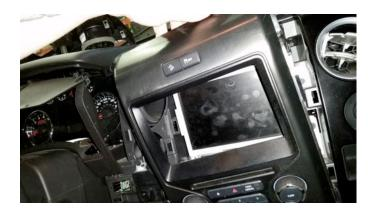
Remove the (4) 7mm bolts holding in the screen/display. Pull screen forward out of dash.
