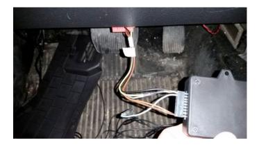
13. Turn the key on to the RUN position, self-programming will start.
