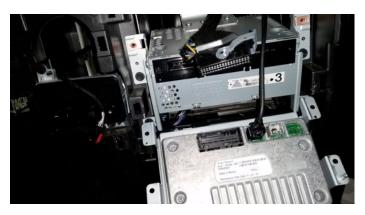
4. Plug the harness into the 2751 module and the male side of the T harness into the back of the screen where the factory harness was just removed. Make sure the handle is locked back in the down position.
