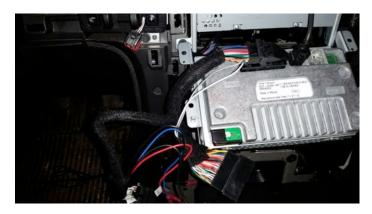
5. Plug the female end of the T harness into the factory harness. Make sure the handle is locked back in the down position.
