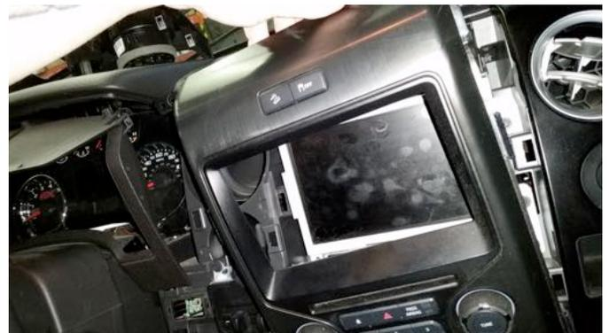
2. Remove the (4) 7mm bolts holding in the screen/display. Pull screen forward out of dash.
