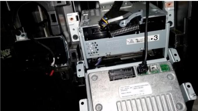
4. Plug the harness into the 2752 module and the male side of the T harness into the back of the screen where the factory harness was just removed. Make sure the handle is locked back in the down position.
