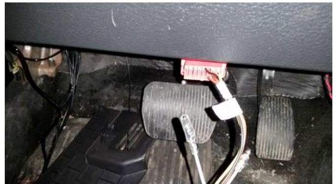
12. Make sure the key is in OFF position. Plug the other end of the harness into the flash module.
