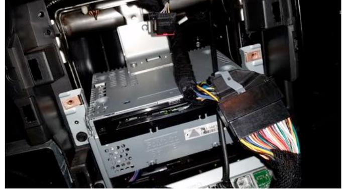
6. Use the red wire for accessory power output and the black for ground output to the camera. The blue, white, and grey with white strip are not used in this install.
