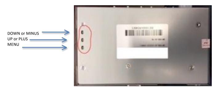
The module box has 3 side keys (highlighted in the red circle above). These are used to tune the picture display and finetune the parking guidelines. Some versions of the module box have the keys labeled on the top of the module.
