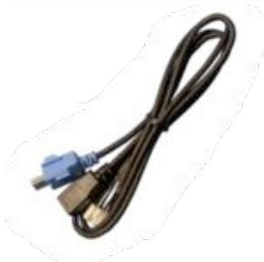
4. Plug the factory blue mini-USB connector into the black, female end of the provided LVDS cable.
