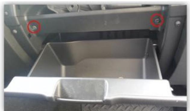
2. GM trucks only: Underneath the glove box you'll find (2x) more additional Torx T15 screws firing upwards. Remove these and pull the glove box
