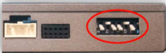
***\*Note: If the dip switches are not configured prior to installation you must remove power to the unit prior to making adjustments to the dip switches. When power is reconnected after the dip switch adjustment the new settings will be stored into memory.***
