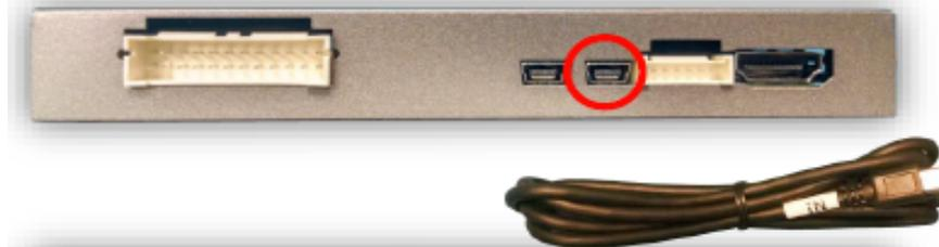
5. Connect the provided **LVDS Output Cable** from the 'VIDEO OUT' connector on the module, directly to the screen LVDS Video port. Make certain the connector is seated firmly.
