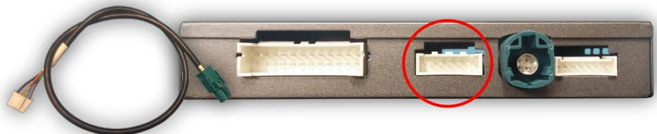
5. Connect the free end of the provided **LVDS Video Cable** (green) back to the factory radio at the appropriate port.
