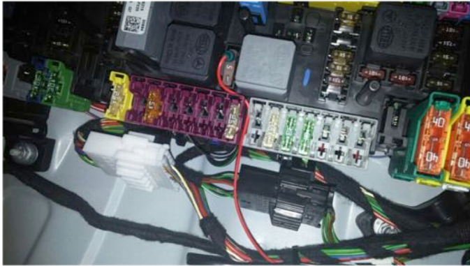
Power connection at fuse panel on passenger floor in CLA
