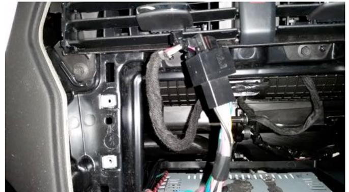
8. Remove (if plugged in) the 4-pin to 6-pin adaptor. It is not need for installation.
