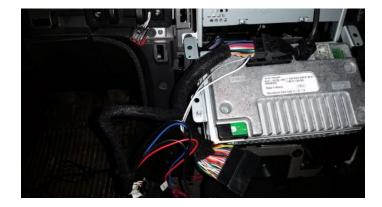
5. Plug the female end of the T harness into the factory harness. Make sure the handle is locked back in the down position.
