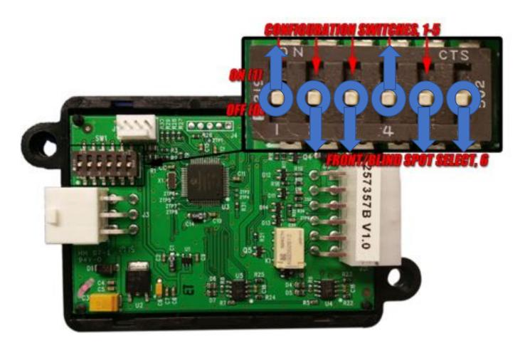
DIP Switches must be set before installation while the module is NOT connected to power for the module to work properly.
