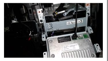
4. Plug the T-harness into the back of the screen where the factory harness was just removed. Make sure the handle is locked back in the down position.
