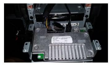
3. Remove the large plug to the left of the screen by lifting the handle like plug.
