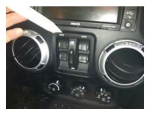
2. Remove the screws holding the radio into the dash.
