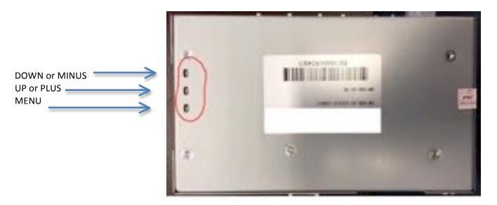
The module box has 3 side keys (highlighted in the red circle above). These are used to tune the picture display and fine-tune the parking guidelines. Some versions of the module box have the keys labeled on the top of the module.
