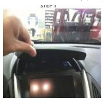
2.Remove console front side trim, by using plastic panel removal tool to release clips. Lift up to remove trim off console.
