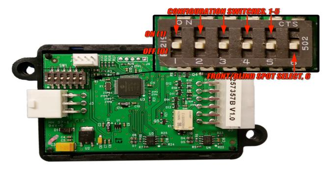
Make sure to adjust the number 6 dip switch to the DOWN/OFF position, when using Brandmotion dual camera interfaces 9002-2780, 9002-2781, 9002-2782 or 9002-2783.
