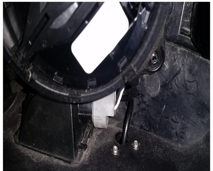
8. Run the camera harness into the vehicle through the door boot.
