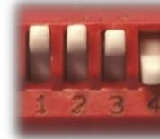
**DIP SWITCH 4: FRONT CAM ACTIVATION**
