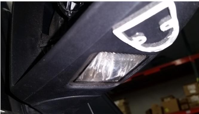
3. Carefully remove the mirror glass from the mirror. Each vehicle is different; consult the vehicles service guide for how to steps.
