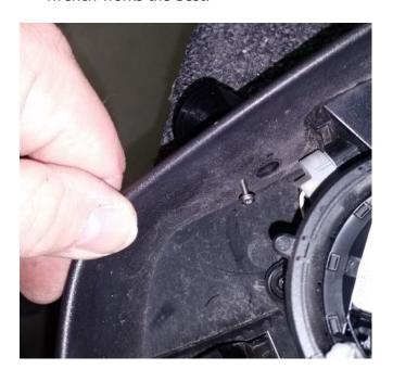
7. Run the camera harness into the mirror and through the arm of the mirror, into the door.
