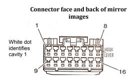
**Step 2:** Insert supplied Orange lead into 16-pin connector cavity 5 and White lead into 16-pin connector cavity 16 until they click into place. If they do not seat initially, use Delphi Terminal Tool 12094429 or a small flatblade watch repair screwdriver to press the terminals fully into the connector. Next, press down on the TPA to lock the terminals.
