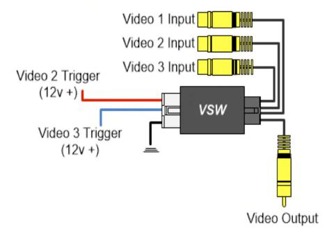
Video 1 Input and Video Output are normally connected (passing video signal) when no
