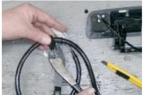
10. Route the gray Camera Harness connector and wiring through tailgate and install supplied handle using an 8mm Socket with the existing hardware.
