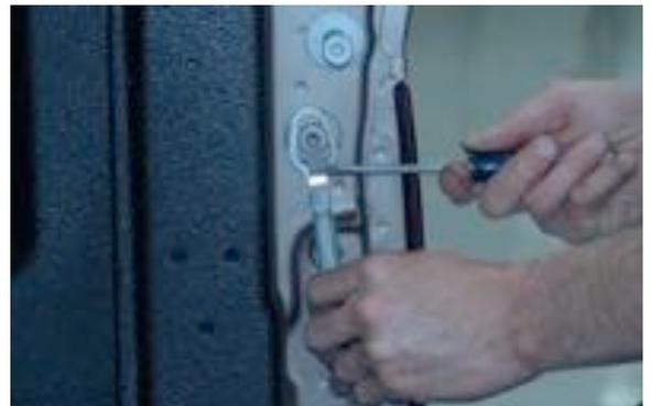
4. Open tailgate about ten degrees and lift right side of the tailgate off the pin. Next, slide tailgate to the right to remove taking care not to damage the paint. NOTE: Tailgate removal and installation requires two people.
