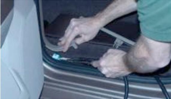
31. Continue to route Chassis Harness along the driver's side front door opening sill area. NOTE: This will be a tight fit, as the supplied Chassis Harness will follow the existing wiring harness.
