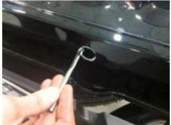
18. Taking care not to damage the Camera Harness, reinstall tailgate by lifting it into place, rotating it down about ten degrees, and sliding it to the left.
