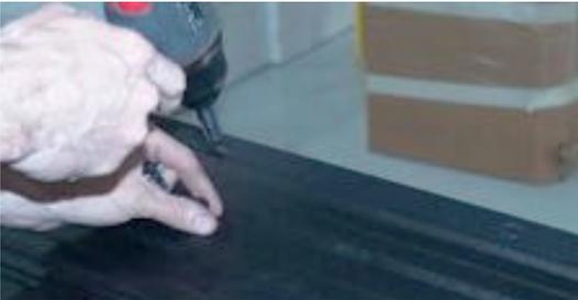
6. Remove nuts attaching handle to tailgate using an 8mm Socket, then remove handle from tailgate. (NOTE: Non-power locking tailgate mechanism shown.)
