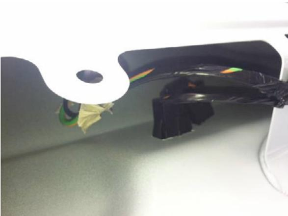
**Step 3: Remove license plate lamp and separate bezel from cover.**
