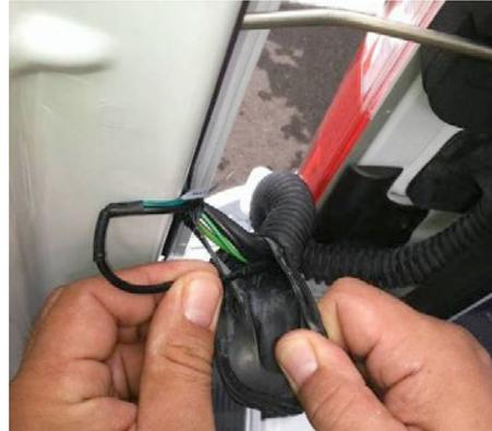
**Step 9: Connect Camera Harness to supplied Chassis Harness.**
