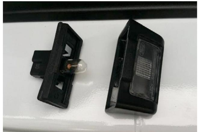
**Step 4: Thread connector end of the camera harness through license plate lamp bezel. Snap supplied camera on license plate lamp bezel.**
