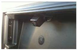
Step 7: Route Chassis Harness RCA plug and Power Harness power connector through rear door grommet.
