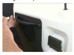
Step 3: Use a Plastic Trim Removal Tool to extract pins from rear passenger door trim panel and remove panel.
