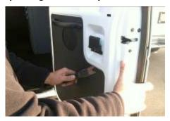
Step 4: Press out the three cut outs in the Camera Mount Gasket, thread Camera Harness through the large opening, and seat gasket to the mount.
