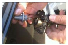
Step 6: Thread connector ends of the Camera Harness through license plate lamp opening and attach Camera using existing scrivets. Remove protective film from the Camera lens.
