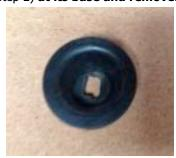
Step 4: Thread Camera Harness video and jumper connector ends through the grommet and through the CHMSL opening. Recommended: Apply a dab of silicone to retain grommet in place and maintain a water tight seal.
