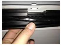
Step 10: Connect Chassis Harness to supplied Video Harness and route beneath headliner and down drivers side A-pillar. (Note: connection is same as shown in Step 8.)
