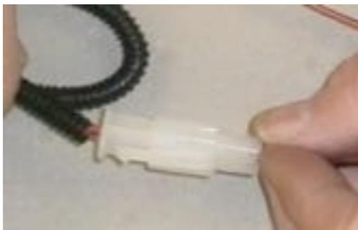
**Step 5: Connect red wire of Jumper Harness to light green CHMSL brake lamp wire (12v+ power) and black wire to chassis ground (Recommended: Solder or T-Taps).**
