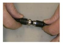
**Step 8: Secure Chassis Harness to existing vehicle wiring**. Avoid binding or otherwise damaging the harness. (Recommended: Wire Ties or Electrical Tape.)
