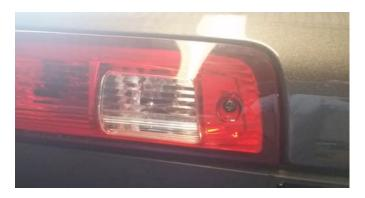
2. Unplug factory connector from the back of the light.
