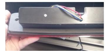
4. Plug the factory connector into the harness connector on the FLTW-7626.
