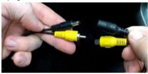
11. Connect Power Harness male RCA connector to RCA located on your Display.
