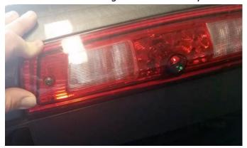
16. Start the screw in the light about a ¼ inch and then put on back of vehicle cab and tighten the screws the rest of the way. (Be sure the foam gasket to set in the correct place). We are not responsible for leaks from around the new lamp.
