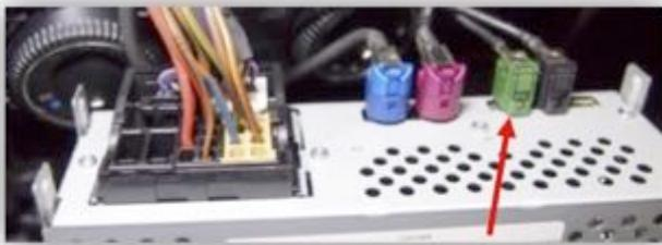
8. Connect the RCA end of the FAKRA to the male to male RCA adapter and other side of the adapter to the yellow video RCA from the camera.
