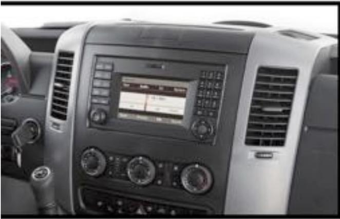
6. Remove the (4) Torx screws from around the radio.
