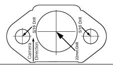
**NOTE:** If self-adhesive Template is missing or damaged, cut out the image above and affix with Masking Tape.
