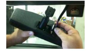
**Step 16: Route Mirror wiring.** Tuck the harness beneath the vehicle headliner and down the A-pillar toward the Chassis Harness which you installed previously.
