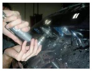
**Step 4:** Drill two 5/16" holes for the camera mounting bolts and one 7/8" hole for the camera harness. Use a Deburring Tool or Round File to smooth edges.
