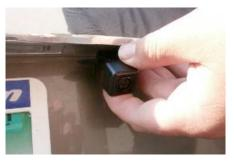
**Step 2:** Peel adhesive backing from supplied Camera Mount Template and apply to the desired location making sure that the camera direction is correct.
