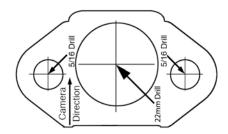
**NOTE:** If self-adhesive Template is missing or damaged, cut out the image above and affix with Masking Tape.
