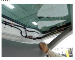
**Step 13:** Remove vehicle mirror. Unplug the 16-pin connector from the rear of the vehicle's mirror, use a T20 Torx bit to loosen the screw securing the mirror, and slide the mirror off the windshield mounting tab.
