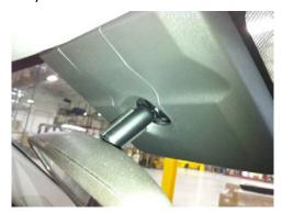
Next, using a Roto Tool remove the striped area of the center cover as shown below. The reworked cover is on the right.
