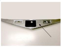
**Step 2:** Peel adhesive backing from supplied Camera Mount Template and apply to the desired location making sure that the camera direction is correct.
