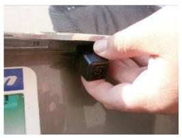
Note: the rear trim of several GM vehicles such as the Chevy Equinox and Cadillac CTS have slight depressions (indicated by the arrow below) where factory installed rear view cameras are mounted. These positions are ideal camera locations.
