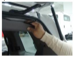
**Step 11:** Route Chassis Harness forward. It may be necessary to remove sill plates, pillar covers, seat bases, side panels, etc. using a Plastic Trim Removal Tool. In some cases, seatbelt bolts must be removed. (**CAUTION:** Any bolts removed for safety devices must be retightened to manufacturer's torque specifications).
