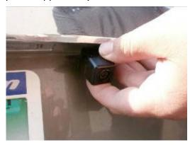
Note: the rear trim of several GM vehicles such as the Chevy Equinox and Cadillac CTS have slight depressions (indicated by the arrow below) where factory installed rear view cameras are mounted. These positions are ideal camera locations.
