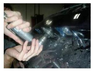
**Step 4:** Drill two 5/16" holes for the camera mounting bolts and one 7/8" hole for the camera harness. Use a Deburring Tool or Round File to smooth edges.
