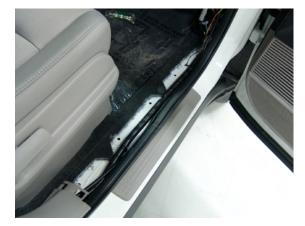
**Step 12: Secure Camera Harness to existing vehicle wiring using supplied Wire Ties**. This will minimize chance of binding or otherwise damaging the harness
