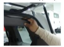
**Step 10: Connect Camera Harness to supplied Chassis Harness**. The optimal location for this junction may occur at the top of the liftgate or the inner edge of the trunk depending on vehicle in which installation is in (Note: Most vehicles may already have existing wires passing through this area; use this route if at all possible).
