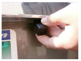
Note: The rear trim of several vehicles have slight depressions (indicated by the arrow below) where factory installed rear view cameras are mounted. These positions are ideal camera locations.
