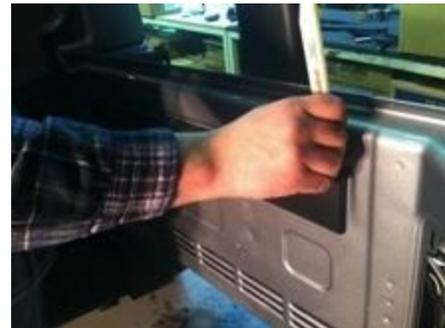
**Step 7:** Pull harness through the rear gate openings.
