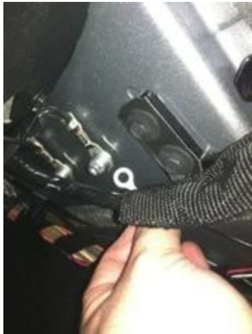
**Step 17:** In the factory wire harness located in the passenger's footwell, locate the White/Gray Reverse signal wire and splice Green Reverse wire from supplied Chassis Harness. RECOMMENDED: Use solder and cover with heat shrink tubing or use T-tabs as an alternate connection method.
