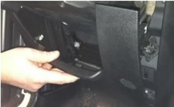
**Step 24:** Remove (2) 7mm bolts on both sides of the steering column.
