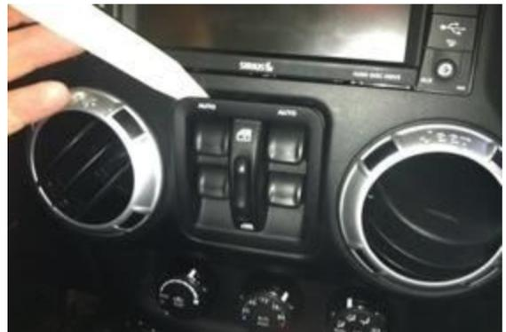
**Step 21:** Disconnect harness from window switches.
