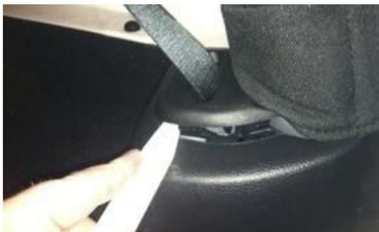
**Step 12:** Using a plastic trim removal tool, remove the rear access panel to expose 10mm bolt, and remove the bolt.
