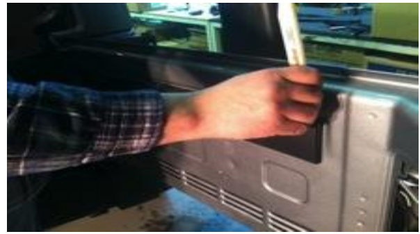
Step 7: Pull harness through the rear gate openings.
