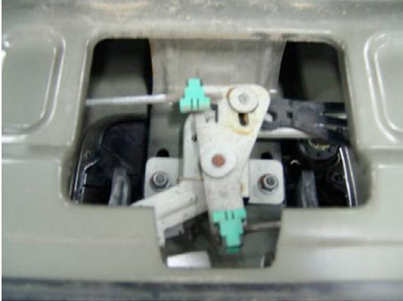
6. Remove lock cylinder from tailgate handle by pulling out wire spring clip (Figure 6).
