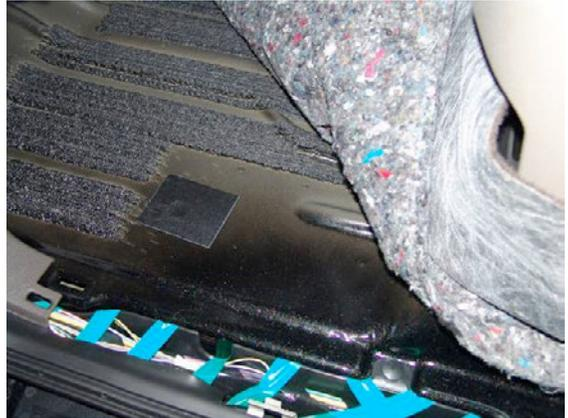
56. Secure Super Duty template number 1008-9100-03 (Figure 39) or secure F150 template number 1008-9100-04 over opening in front of driver's seat (Figure 40).
