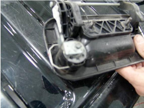
7. Install lock cylinder into supplied tailgate camera handle with by pushing cylinder into handle. Secure the cylinder with the wire spring clip.
