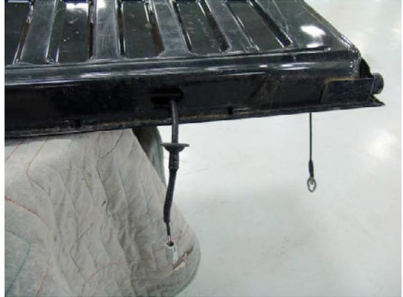
9. Install supplied tailgate handle camera into tailgate by tightening two nuts with 10mm socket (Figure 8).
