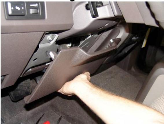
41. Remove the driver's side knee bolster reinforcement by removing the four M8 screws (Figure 28)
