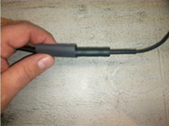
66. Heat and seal the connection between the chassis harness and camera (Figure 50).
