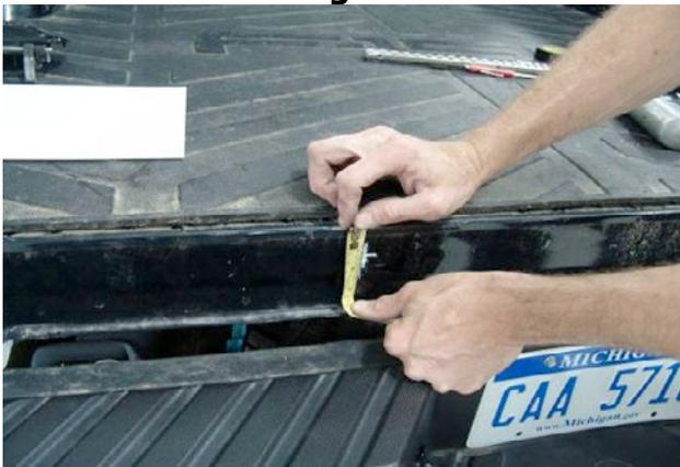
3. Center punch the mark and drill a pilot hole. Next, cut a 1/2 inch opening with a hole saw (Figure 3).
