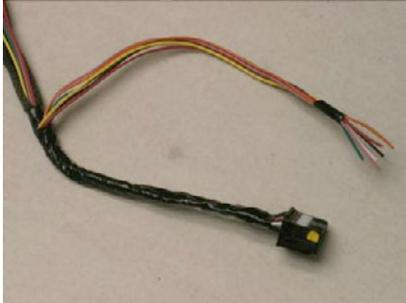
27. Consulting the Connector C911 pinout diagram opposite, splice the seven wires to the vehicle mirror harness wires according to Diagram A1.
