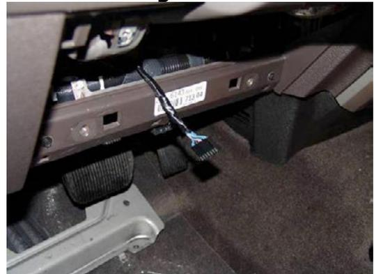
43. Place the mirror circuit board as shown (connector facing forward and towards the bottom). Secure the circuit board to the existing cross dash harness with the two supplied long wire ties (Figure 30)
