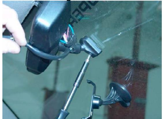
**NOTE:** On some models without screws, Mirror Removal Tool # OTC8200 is required.
