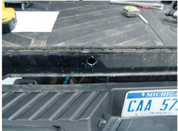
4. Clean the rough edges of the opening with a deburring tool. Apply supplied Z-tech with a small brush (Figure 4). Reinstall tailgate.
