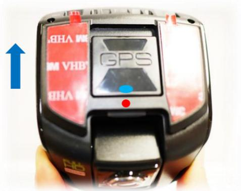
Press the bracket and slide it upwards until it
