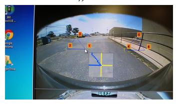
11. After you have aligned the triangles, click on APPLY AVM at the top of the screen. You may receive an error message if one of the triangle points is hidden by the vehicle body or "out of view" by the software program. Click OK to acknowledge the message and continue. (*There are no banners in the pictures, pictures are for instructions only*).
