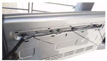
11. Run the camera harness through the factory cloth door boot, use a long zip tie or a fish tape.
