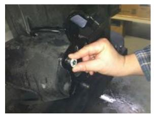
4. Run the harness into the rear gate through the factory gromet.
