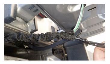
12. Finish running the harness to the front glove box area on the passenger side of the vehicle.
