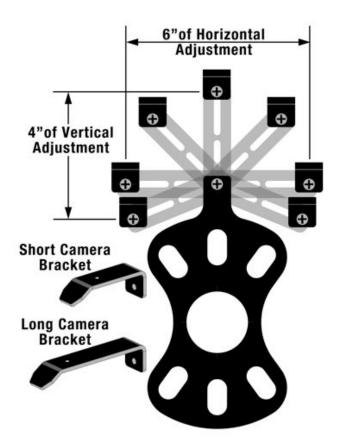
**Note:** Short Bracket has been designed for Factory offset wheels. Use the Long Bracket for wheels with larger offsets.
