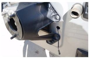
5. Run rear camera harness through top hole of tire carrier.
