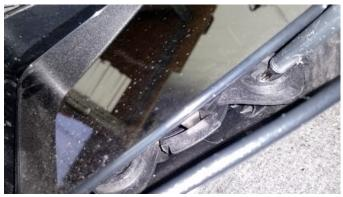
12. Remove the mirror glass by gently lifting on the tabs.
