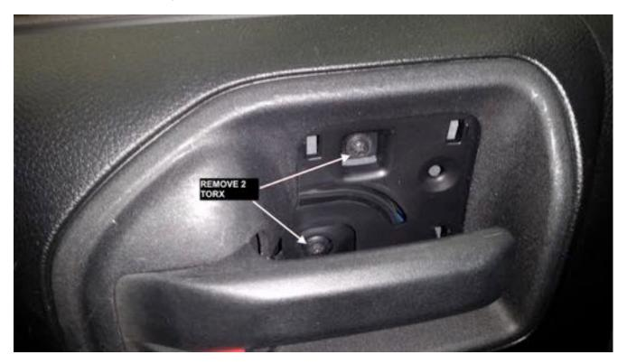
4. Remove the inter trim on the pull handle to gain access to the two screws behind the trim.
