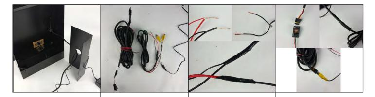
5.1- Feed video harness from backup camera and power supply cord through top of metal plate as shown. 5.2- Locate power/video harness for camera and monitor. Strip ends of loose red and black wires for both. Do not strip brown wire. 5.3- Secure positive and negative connections between harnesses. Remove end of power supply, strip wires, then secure positive and negative connections. (on power supply, gray dashed line is negative)
