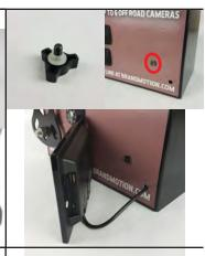
6.4- Slide plastic washer over bolt, insert through back of display at location marked, then loosely attach metal square. Feed video cable through lower hole. Slide monitor over metal square and gently tighten.
