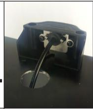
4.1- Center the camera on the top of the display, allowing the front of the camera to slightly overhang.
