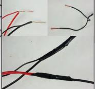
7.3- Secure positive and negative connections between harnesses. Remove end of power supply, strip wires, then secure positive and negative connections. (on power supply, gray dashed line is negative)
