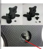
6.3- Remove metal square, retaining collar, and bolt from stand. Use pick to dislodge retaining collar from bolt.
