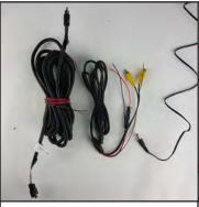
7.2- Locate power/video harness for camera and monitor. Strip ends of loose red and black wires for both. Do not strip brown wire.
