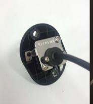
5.2- Attach bracket to camera housing.
