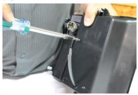
Step 20: From the topside insert the remaining (2) 1/4" flat head screws through the substrate and into the modules. Unscrew the other (2) previously inserted ¼" flat head screws and repeat steps 17 through 19. Then replace the remove ¼" flat heads screws.
