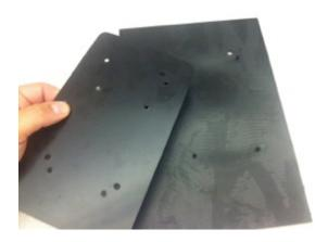
Step 12: Align LED holes and insert mats crosshair locators through substrate hole to insure proper alignment.
