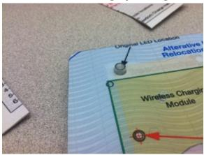
Step 7: With trimmed template placed on top of Freedom Charge module check for correct fit in vehicle. Make any trim adjustment(s) needed to template to achieve perfect fit.
