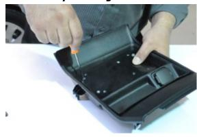
Step 18: Remove Charging Module and Drill 3/18" holes at the previous 2 marked locations.
