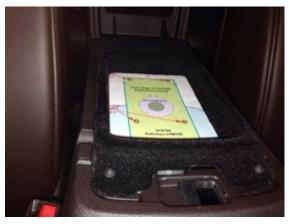
Step 33: Drill (4) 1/8" holes in marked mounting hole locations and (1) 1/4" hole for LED. Also drill the (4) 3/16 holes for the non-skid mat location crosshairs.
