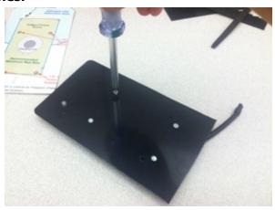
Step 16: Place new assembly into vehicle tray or bin to mark ½" hole location required for power connector to pass through. Drill 1/2" hole in marked location.
