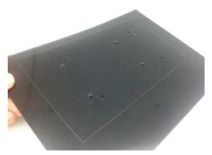
Step 10: Substrate can be trimmed with scissors. Be careful to cut right on the scribed line. Again check fit in vehicle.
