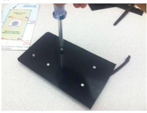
Step 25: Place new assembly into vehicle tray or bin to mark ½" hole location require for power connector to pass through. Drill ½" hole in marked location.
