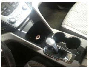
Step 2: If chosen location has mat, remove to add in making template otherwise carefully cut template to fit. Always start larger and slowly trim down to ensure best fit. Make sure to account for draft as the Freedom Charge Module is about ½" think. If using the Drop-In method of attachment a mat at a bottom of a drafted bin may be slightly smaller than your final substrate and mat solution.
