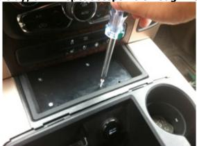
**Step 29: Install Non-Slip Freedom Charge Mat to Wireless Charging Module.** Place the 4 locator pins in corresponding holes.
