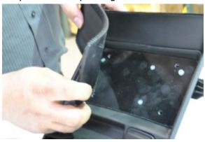
**Step 22: Firmly press Mat around LED.**
