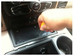
Step 27: Remove Charging Module and Drill 1/8" holes at the previous 2 marked locations.
