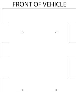
**Step 8:** Place the substrate on the top of the FDMC tray with the LED Hole facing the front of the vehicle. Push the LED into the hole 1/4 past the substrate. Attach to FDMC tray using the following screw options:
