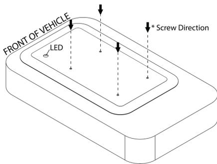
If metal plate **IS USED:** use 1" long black screws to attach substrate, and mount the metal bracket:
